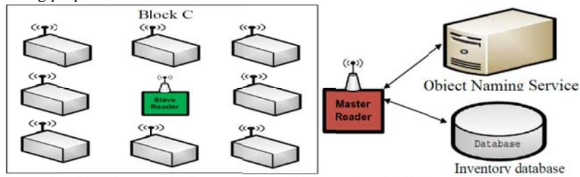
Fig 3 (a) Block Structure (b) Communication of Master reader with ONS and Inventory database
