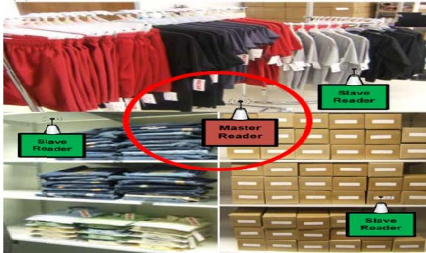
Fig 5: Retail shop with different products placed different blocks and monitored by their Slave Readers
